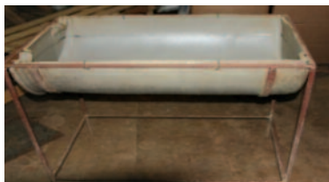
Figure 12: Dip tank made from food-grade plastic and supported on a metal stand
