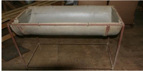
Figure 12: Dip tank made from food-grade plastic and supported on a metal stand
